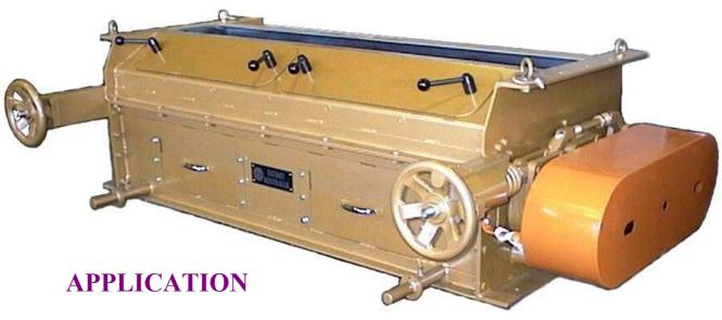
The Satake Pellet Crumbler is used to reduce pellets produced on a press to "crumbles". The pellets are ground between two fluted rolls that are fully adjustable allowing accurate particle size reduction.
