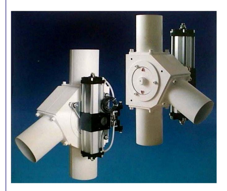
The diverting valve type "VDM" is used in the pneumatic conveying lines both in negative than and positive pressure. It consists of a cast iron slide controlled by a rotary pneumatic cylinder with magnetic end switches. The lateral covers are made in bronze, the air seals in anti-wear material (Teflon). The valve is equipped with joint-pipes in different diameters to satisfy all the needs of the customer.
